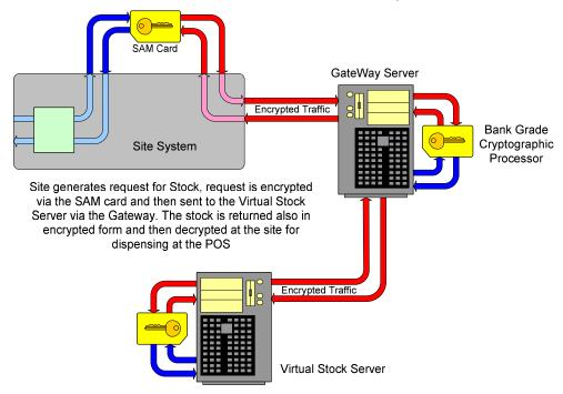
There is no problem interfacing to virtually any Point of Sale system as the Recast system does not integrate with the Point of sale but sits between the Point of Sale computer and the peripheral units that are connected.
